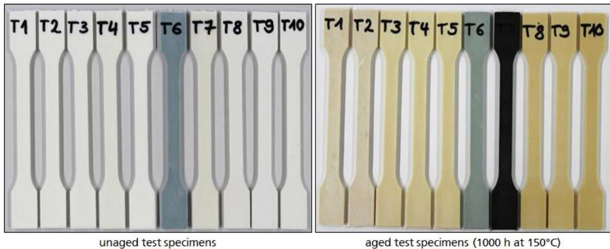
*Figure 2: tensile test specimens in unaged (left) and aged state (right)*
