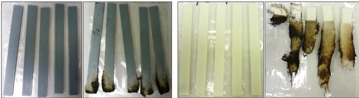
*Figure 1: 3 mm thick test specimens before and after the UL94 testing, no classification (left) and "Vo" classification (right)*
